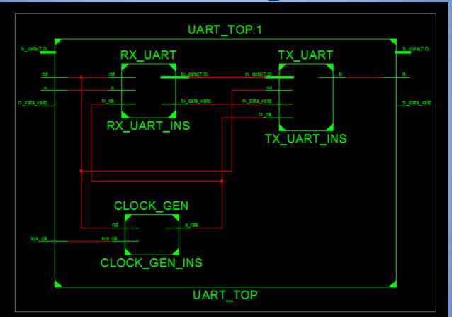
In this case, TX\_DATA and TX\_DATA\_VALID has no use as the outputs of receiver are connected directly to inputs of transmitter.
