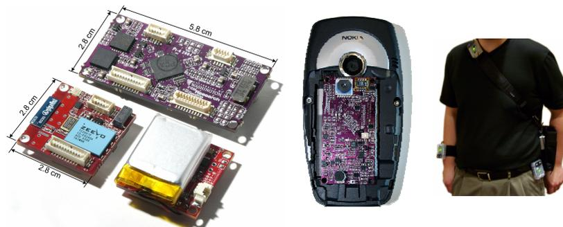
**Figure 1.** The multimodal sensor board (*top*), a Bluetooth iMote (*lower left*), and USB rechargeable battery board (*lower right*). A Nokia 6600 series phone with a sensor board on the back for scale (*middle image*). The data collection setup consisted of three sensor boards and a small Vaio Notebook for data logging (inside the pouch on the user’s right side)
