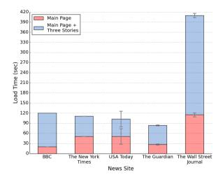
**Fig. 5.** The average loading time for news sites using CovertCast over YouTube. The time to load the site's main page and the time to load three news articles were measured. Each site was loaded five times. The variance for *USA Today* is due to non-determinism in Ghost.py deciding when a page is fully loaded.
