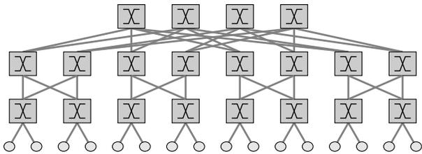
**Figure 9: Testbed used in our experiments** has 16 servers, each with 1Gbps access link bandwidth, interconnected with a FatTree topology comprising 20 PICA8 switches. Each switch supports priority queuing with 8 distinct levels.
