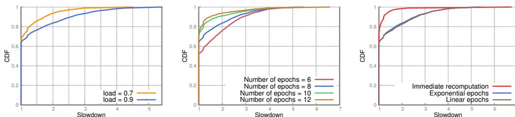
**Figure 7: Sensitivity analysis of Sincronia performance** over varying network load (left), varying number of epochs before resetting the time horizon (center) and varying epoch mechanisms (right). More discussion in §5.2.
