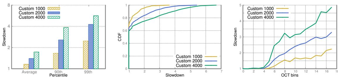
**Figure 6: Sincronia evaluation results for the online case.** (left, center) For the evaluated workloads, Sincronia achieves performance within  $1.7\times$  on an average and  $5.7\times$  at high percentiles when compared to an unloaded network; (right) Coflows with larger sizes observe larger slowdown in online version of Sincronia. More discussion in §5.2.
