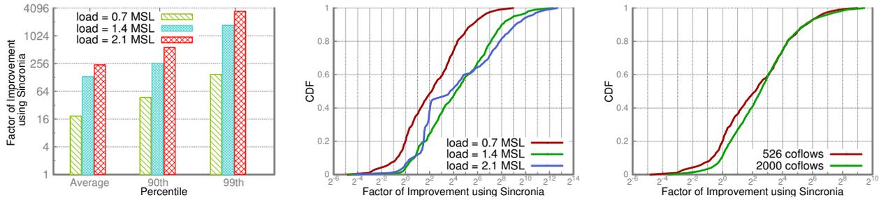
**Figure 8: Evaluation results for Sincronia implementation on top of TCP over our testbed in Figure 9.** Sincronia when implemented on top of TCP/DiffServ significantly improves coflow performance when compared to coflow-agnostic TCP both on an average and at high percentiles (left), and maintains these improvements across varying network loads (center) and trace sizes (right). More discussion in §5.3.
