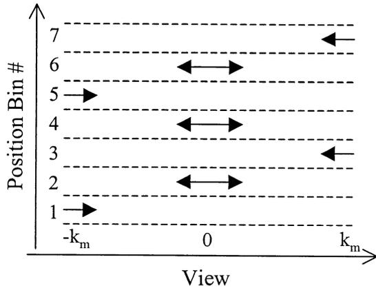
Fig. 2. k-space sampling for modified PAWS algorithm. The arrows indicate the sampling directions in k-space. The k-space center is sampled at every other position bin to ensure smooth motion distribution in k-space for the final reconstructed data.
