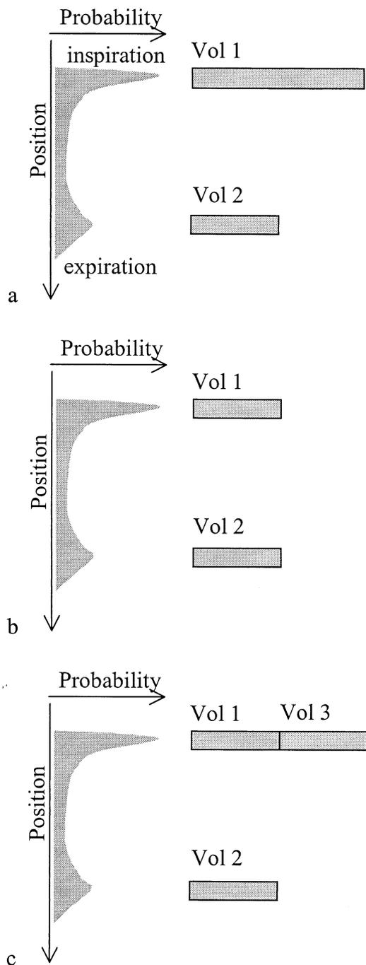
Fig. 1. SMV algorithm simultaneously using 2 gating windows at the two peaks of histogram of motion (respiration as a specific example here) to acquire (a) 2 volumes with their sizes proportional their corresponding histogram peak heights, (b) 2 volumes of equal size, and (c) three volumes of equal size.
