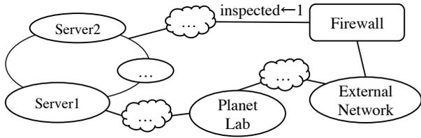
**Figure 7: An example where packet transformations allow convenient checking of firewall policy. Solid lines are network links; text on the links represents a transformation constraint to express the invariant. Clouds represent omitted components in the network.**
