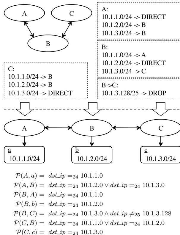
Figure 3: An example of a 3-node IP network. *Top*: Network topology, with FIBs in dashed boxes. *Bottom*: graph used to model network behavior. Ovals represent networking equipment; rounded rectangles represent special vertices such as destinations, labeled by lower case letters. The lower half of the bottom figure shows the value of  $\mathcal{P}$  for each edge in the graph.
