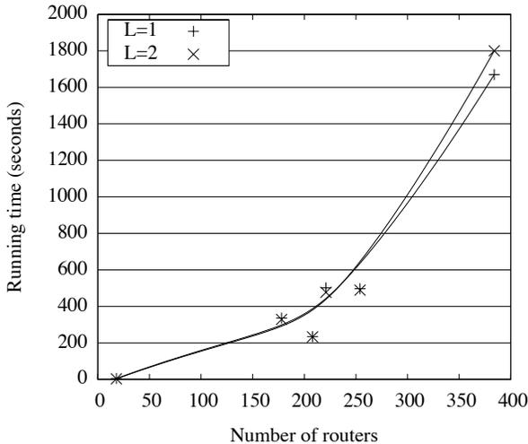
Figure 13: Scalability results of the loop-free forwarding invariant on six AS networks from [36].  $L$  is the parameter to control the complexity of FIBs. Dots show the running time of the invariant for each network. Solid lines are fitted curves generated from the dots.
