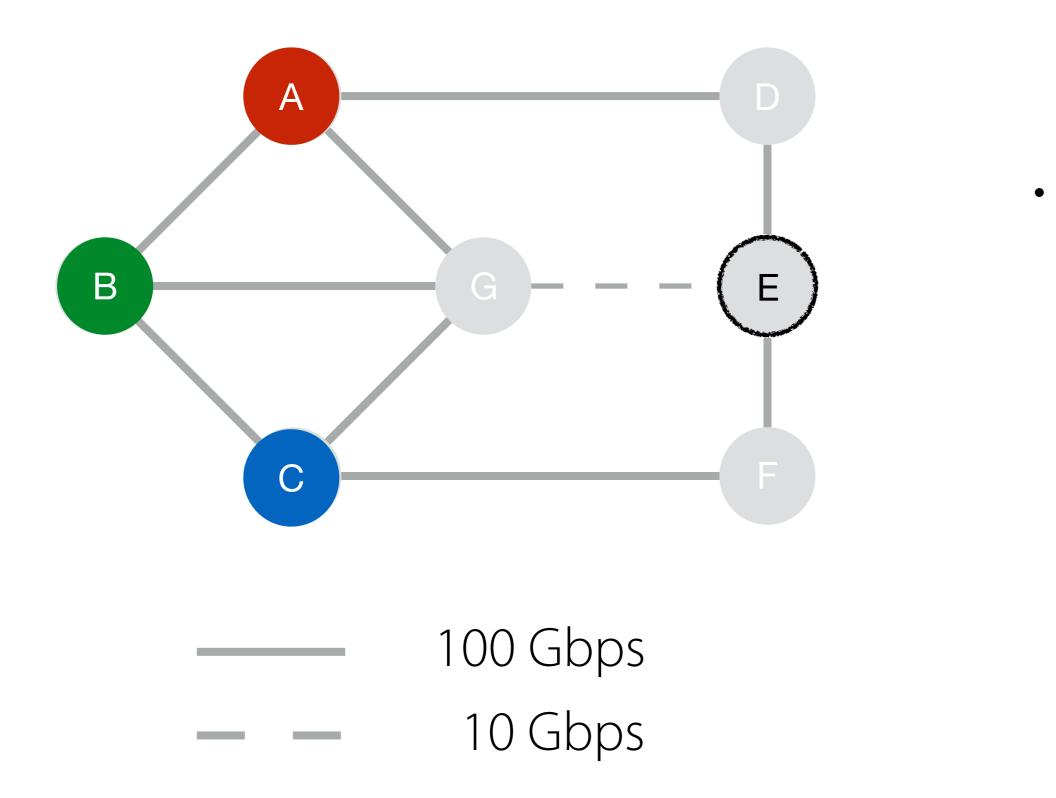
• Traditional approaches to routing based on shortest paths (e.g., ECMP, KSP) are generally not capacity aware
