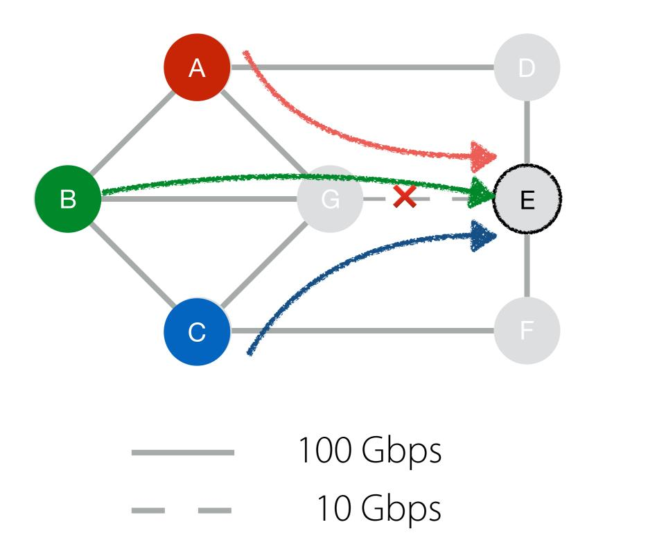
• Traditional approaches to routing based on shortest paths (e.g., ECMP, KSP) are generally not capacity aware
