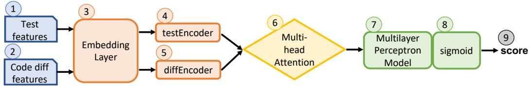
Figure 3: Architecture overview of our ML-based RTS models.
