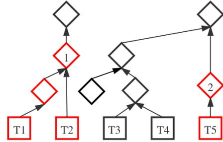
**Figure 1: An example dependency graph: diamonds are code entities (e.g., modules/classes/methods) and squares are tests. An edge  $A \rightarrow B$  means that  $A$  directly depends on  $B$ . In this figure, entities 1 and 2 changed (colored red). Tests T1, T2, and T5 transitively depend on entities 1 and 2 (also colored red), so they are selected.**
