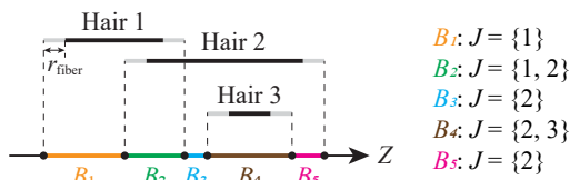
Figure 8: Hybrid approach: discretizing the Z dimension based on the two endpoints (i.e., z_{j,1} - r^{\text{fiber}} and z_{j,2} + r^{\text{fiber}} ) of each hair-type fiber j . In this example, there are three hair-type fibers that yield a discretization of five bins B_1, B_2, \dots, B_5 . The set of active fibers \mathcal{J} remains constant in each bin.
