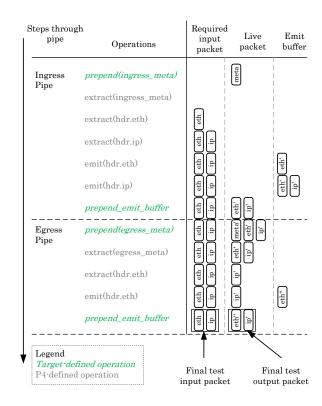
(a) Extern sequence manipulating Ethernet and IPv4 headers.
