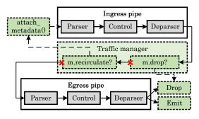
(b) P4Testgen control-flow. Dashed segments are target-defined. ✗ is false Figure 5: P4Testgen's pipeline control flow.
