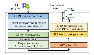
Figure 1: The P4Testgen test case generation process.
