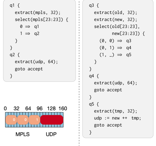
Figure 1. Reference (q1, q2) and vectorized (q3, q4, q5) parsers for MPLS and UDP headers (depicted inset).
