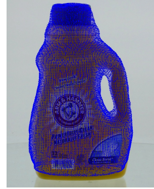
Fig. 8. The 3D mesh is projected onto one of the Canon images.
