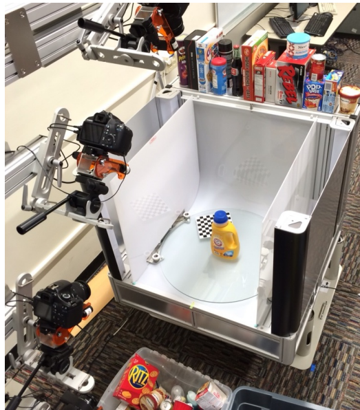
Fig. 1. Our data-collection system. We place the object near the center of the turntable, and our software takes care of the rest. Note the chessboard on the turntable to merge clouds as the turntable moves. Sample objects from the dataset can be seen sitting on top of the Ortery Photobench.
