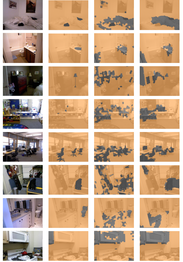
Fig. 5: The columns represent the original RGB image, ground truth, unary, and CRF output respectively from our approach in the NYU V2 dataset. Each row represents a case study for a particular object interest. From top to bottom, the objects of interest are Clothes , Sink , Lamp , Box , Chair , Bag , Toilet , and Cabinet respectively.
