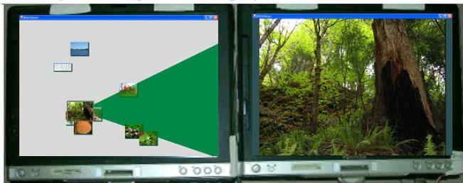
Fig. 4 Gallery: The right tablet displays a full-screen view of an image that the presenter selects on the left tablet.
