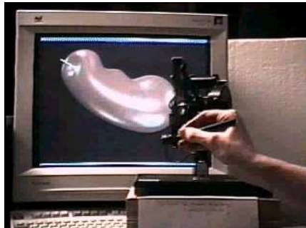
Figure 1.10. : Photograph of simulation in use: Users were able to push, slide and pull on the surface of the model using a point-like manipulum.
