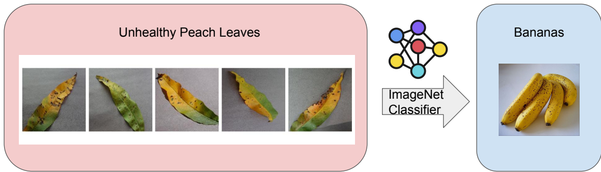
Figure 1: Predictions by an ImageNet classifier on five unhealthy peach leaves. While the classifier is not trained to classify unhealthy peach leaves, it recognizes all of them as bananas. The predictions are not semantically correct, but they correctly group unhealthy peach leaves into a single cluster. This indicates that the pseudo-labels by the classifier contain valuable signals that could be used for bootstrapping new perception models.
