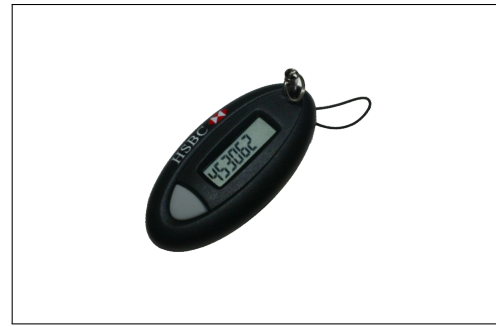
Fig. 2. Hardware tokens used in banking. These devices store secret information into a tamper-resistant hardware. One on the left, has device with screen and keyboard; on the right, a device with screen and just one key.
