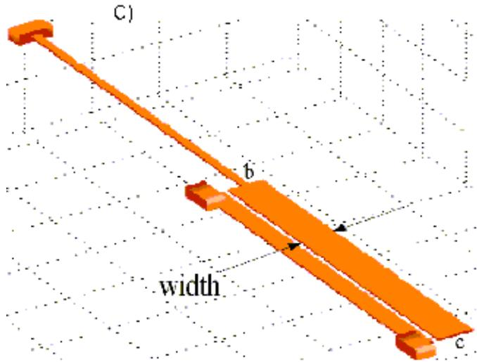
Figure 1: electrostatic beam actuator
