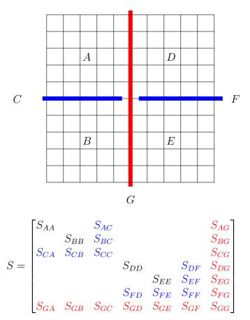
Figure 1: Nested dissection on a square mesh. We first cut the graph in half with the red separator G, then further dissect the halves with the blue separators C and F. Nodes in A, B, D, and F are only connected through these separator nodes, which is reflected in the sparsity pattern of the adjacency matrix S when it is ordered so that separators appear after the things they separate.
