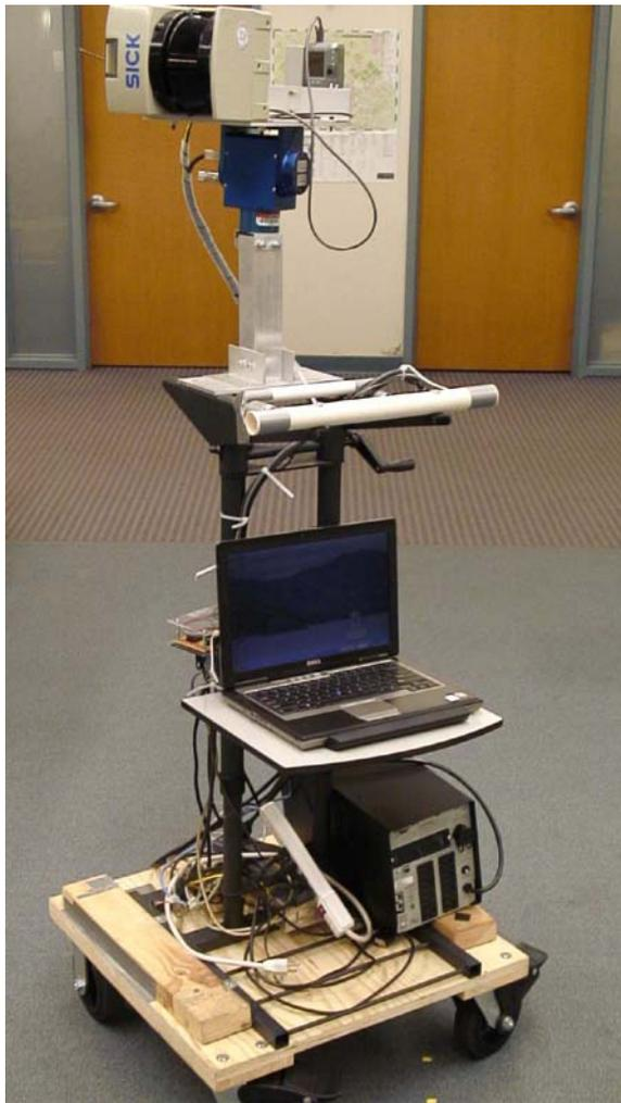
**Fig. 7** The 3-d scanner used for collecting images and the corresponding depthmaps
