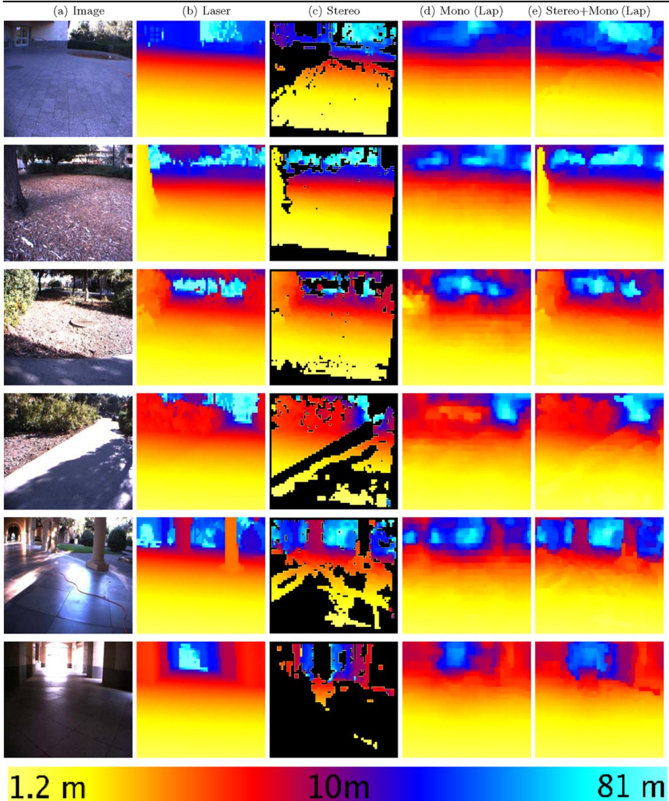
**Fig. 13** Results for a varied set of environments, showing one image of the stereo pairs (*column 1*), ground truth depthmap collected from 3-d laser scanner (*column 2*), depths calculated by stereo (*column 3*), depths predicted by using monocular cues only (*column 4*), depths pre-
