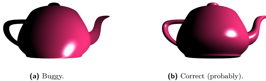
■ Figure 1 Output from a buggy and corrected implementation of the Phong lighting model. The difference is obvious now but was hard to detect without a ground-truth comparison.
