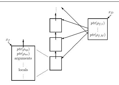
Figure 7: Snapshot of the stack and display during the execution of a translated program.
