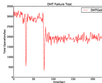
Figure 10: While a stream of OrderedGet requests are performed, the DHT is forced to recover from failures at times 30 and 60.
