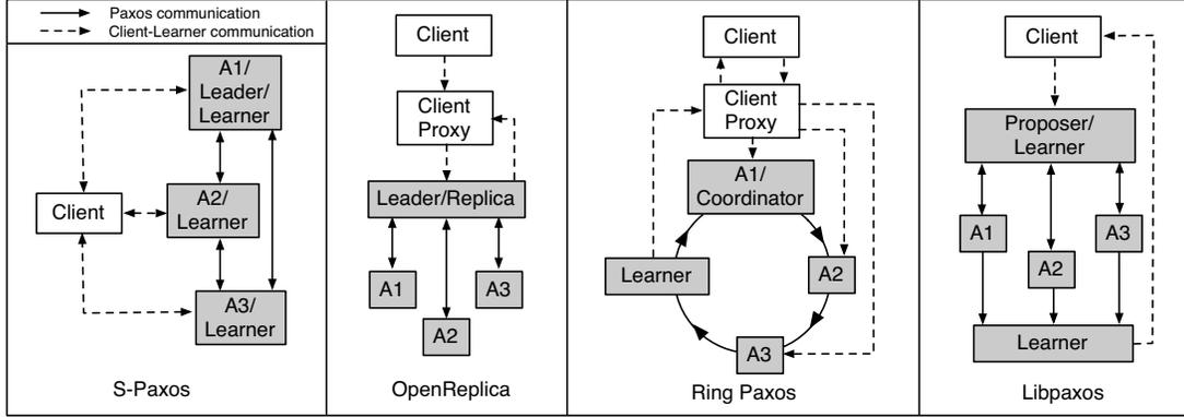
Fig. 1. The communication pattern and architectural differences among the four libraries as deployed in the experiments;  $f$  is equal to one; the picture preserves the terminology of the libraries; dashed lines show the communications between the learner/replica and the clients; in all the libraries the learner/replica sends the responds back to the client; in S-Paxos and OpenReplica clients send their requests to the nodes that also assume the learner/replica role.
