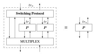
The switching protocol affects the traces  $tr_1$  and  $tr_2$  in two ways: first, they will be merged in some way, and second, the order of some events in the merged trace may be modified due to the effects of layering.
