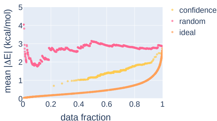
Figure 8. Mean barrier height of React-OT with different methods for adding confidence data. Yellow corresponds to the confidence model used in the main text. Pink corresponds to random selection, giving mean errors oscillating around the overall model performance. Orange corresponds to the ideal case, where the lowest error data point is always selected as the data fraction increases.
