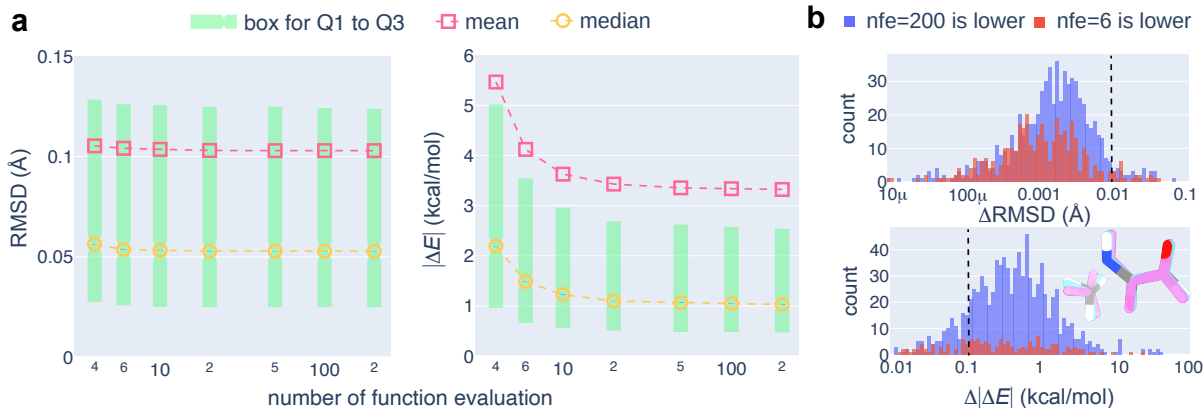
Fig. 3 | Performance of React-OT with respect to the number of function evaluation (nfe). a. Distribution of RMSD (left) and |\Delta E_{\text{TS}}| (right) between the true and generated TS on 1,073 set-aside test reactions, where the mean is shown in pink and median is shown in yellow. The first and third quarter is bounded by a green box. b. Absolute difference in RMSD (top) and |\Delta E_{\text{TS}}| (bottom) for generated structures at nfe=6 and nfe=200. Structures where nfe=200 gives better quality is shown in blue, otherwise shown in red. A threshold below which the comparison is not chemically meaningful is shown (dashed vertical line). Reference TS structure and React-OT generated structure at nfe=6 (pink) and nfe=200 (skyblue) for a select reaction. Atoms in the reference TS are colored as follows: C for gray; N for blue, O for red, and H for white.
