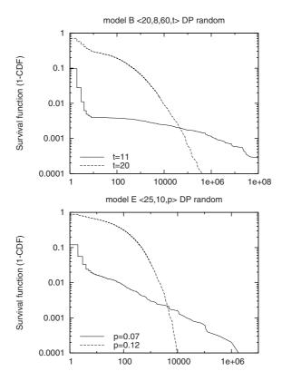
**Fig. 6.** Heavy-tailed and non-heavy-tailed regimes for instances of (top) model B  $\langle 20, 8, 60, t \rangle$ , using DP-random (DPLL procedure with static variable ordering and random value selection) and (bottom) model E  $\langle 25, 10, p \rangle$  using DP-random.
