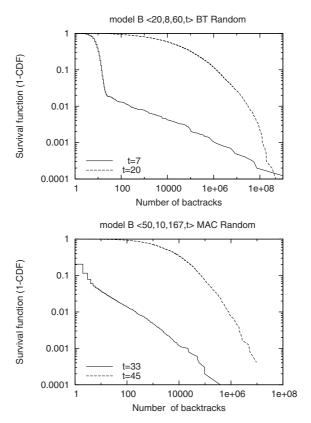
Fig. 5. Heavy-tailed and non-heavy-tailed regimes for instances of model B: (top)  $\langle 20, 8, 60, t \rangle$ , using BT-random, (bottom)  $\langle 50, 10, 167, t \rangle$ , using MAC-random.
