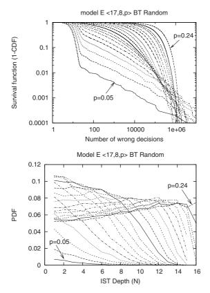
**Fig. 4.** The progression from heavy-tailed regime to non-heavy-tailed regime: (top) survival function of runtime distribution; (bottom) probability density function of the corresponding inconsistent sub-tree depth (ISTD) distribution.
