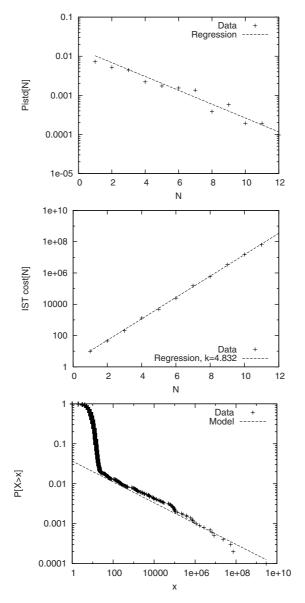
**Fig. 7.** Regressions for the estimation of B1=0.015, B2=0.408 (top plot; quality of fit  $R^2=0.88$ ), and k=4.832 (middle plot;  $R^2=0.98$ ) and comparison of lower bound based on the theoretical model with empirical data (bottom plot). We have  $\alpha=B_2/\ln(k)=0.26$  from our model;  $\alpha=0.27$  directly from runtime data. Model B  $\langle 20,8,60,t\rangle$ , using BT-random.
