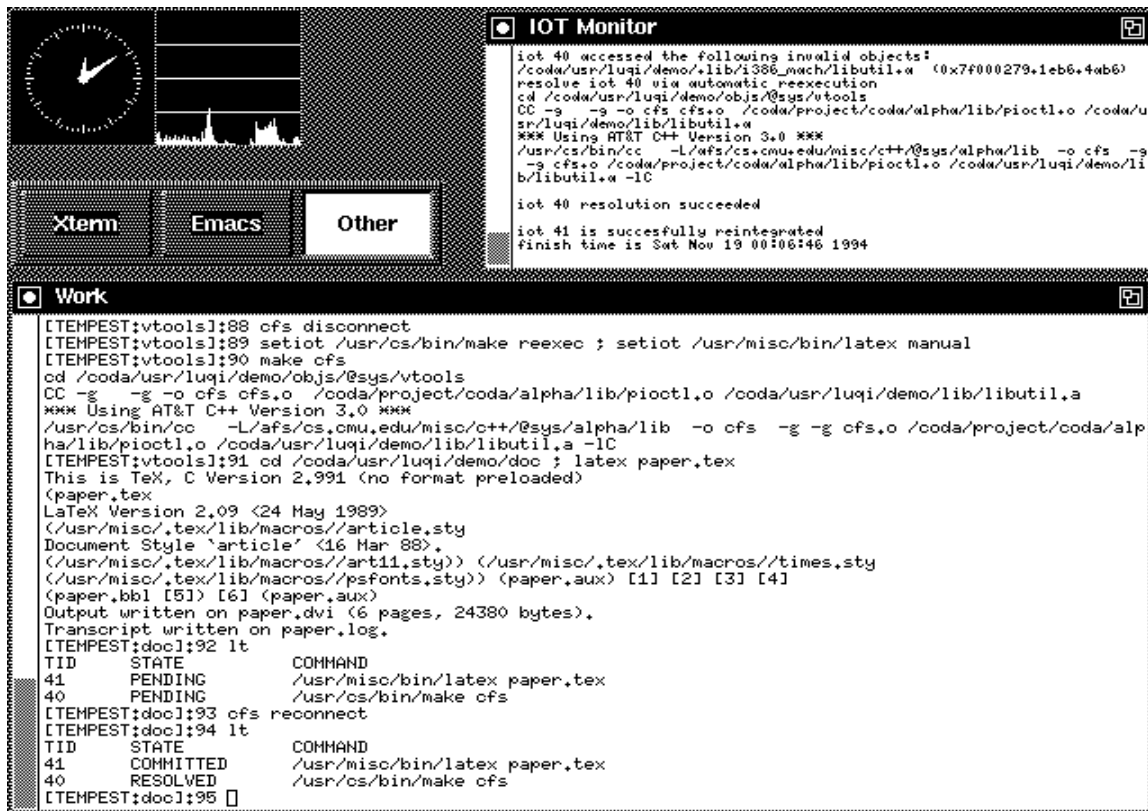
The work window displays the process of disconnecting the client, setting make and latex as transactions in the special IOT shell, executing a make transaction and a latex transaction, reconnecting the client, and checking transaction status using the lt (list transaction) command. At reconnection time the make transaction is invalidated because the linked library libutil.a was updated on the servers. The IOT monitor window shows the automatic re-execution of the make transaction and the committing of the latex transaction.
