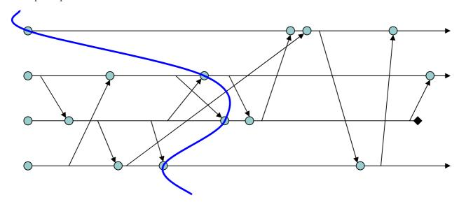
The thick blue line here represents the current best recovery line. The diamond indicates that the third processor failed at that point.
