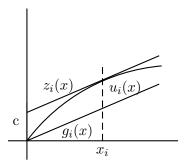
**Step 1:** Define  $z_i(x) = u_i(x_i) + (x - x_i)u'_i(x_i)$  where  $x_i$  are the values of the individual bandwidths in the Nash. We use  $z_i$  to be the new utility function of all users. i
