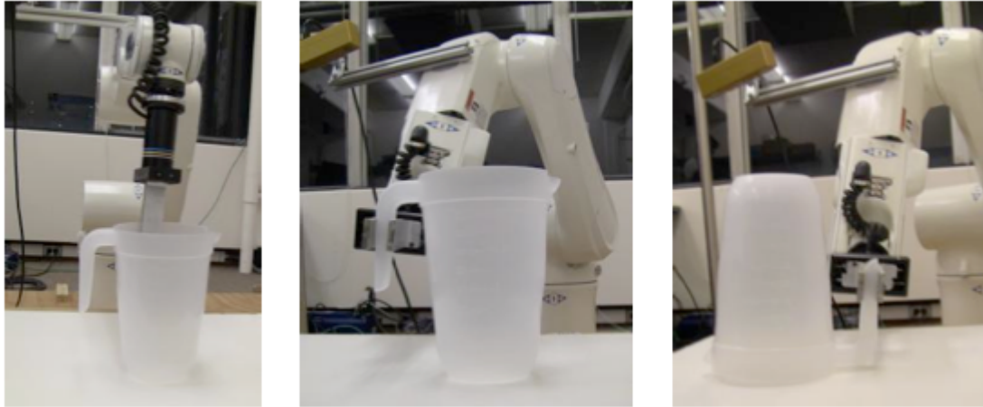
Figure 1: If the intent is to flip the cup over, the grasp on the left will result in failure due to the gripper colliding with the ground. A better grasp is shown in the middle picture where the transformed position (right) is also a good grasp.
