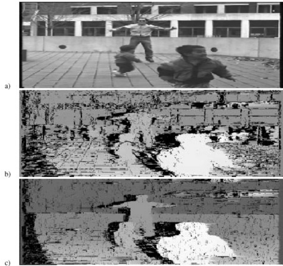
Fig. 12. Results of two stereo algorithms on Figure 1. (a) Original left image. (b) Cox et al. algorithm[ 14], and (c) the algorithm described in this paper.
