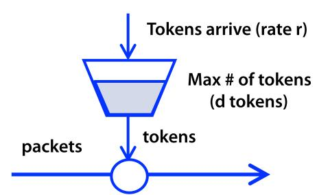
A leaky-bucket shaper for each flow or traffic class
