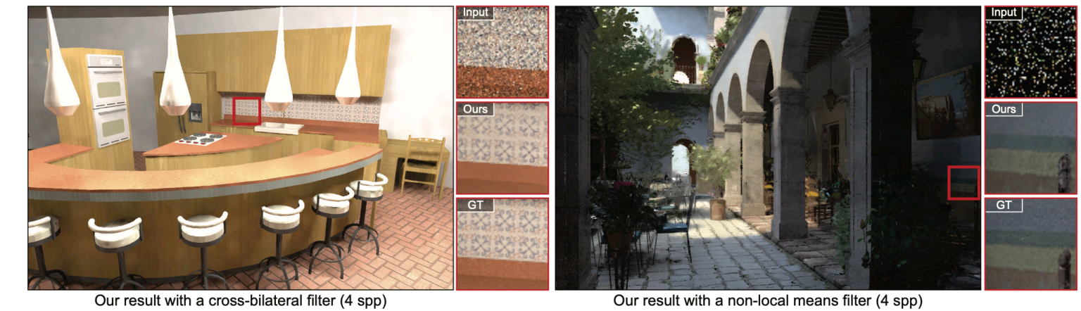
Figure 1: We propose a machine learning approach to filter Monte Carlo rendering noise as a post-process. In our method, we use a set of scenes with a variety of distributed effects to train a neural network to output correct filter parameters. We then use the trained network to drive a filter to denoise a new MC rendered image. We show the result of our approach with a cross-bilateral filter for the KITCHEN scene ( 1200 \times 800 ) on the left and with a non-local means filter for the SAN MIGUEL HALLWAY scene ( 800 \times 1200 ) on the right. Both of these scenes are path-traced and contain severe noise at 4 samples per pixel (spp). However, our trained network is able to estimate the appropriate filter parameters and effectively reduce the noise in only a few seconds. Note, the tonemapping of the insets has been adjusted for best visibility. Scene credits: KITCHEN – Jo Ann Elliott; SAN MIGUEL HALLWAY – Guillermo M. Leal Llaguno.
