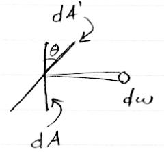
If we call the inclined surface area  $dA'$  and continue to call the perpendicular surface area  $dA$ , then  $dA = dA' \cos \theta$ . So the radiance can be written
