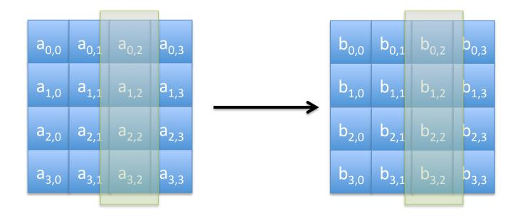
Each column is transformed by a complex (but fixed) algebraic equation that takes input from all four bytes and incorporates them into each output byte
