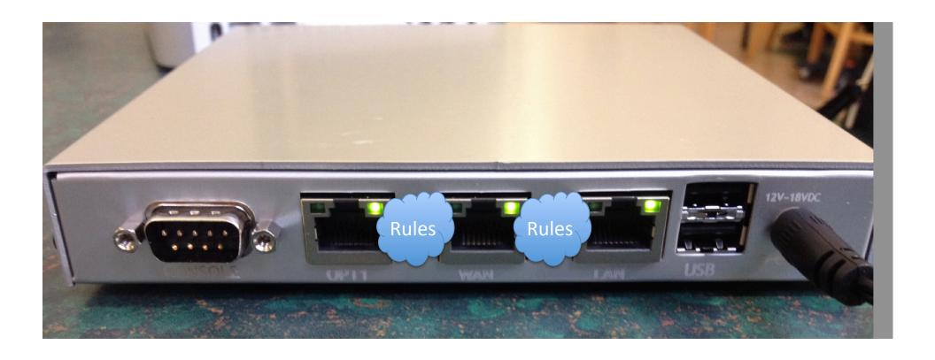
(This is Netgate M1N1Wall – low-cost, low-power open source firewall using FreeBSD/pfSense. Runs on AMD Geode cpu.)
