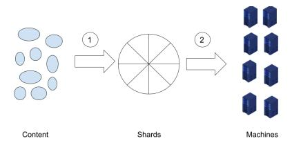
In this graphic, the Akamai-hosted content is on the left. In step ① Akamai hashes the key for each content item, placing the key-value pair along the ring at the numerical location that the hashed value takes us to (the numbers wrap at the top). The ring is split into shards – our graphic shows eight shards. Step ② is managed by the team Anna works on, and involves storing the DHT into the servers, which are shown on the right. Select the statements that are correct.
