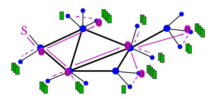
Overcast is application-level multicast in an overlay network.
