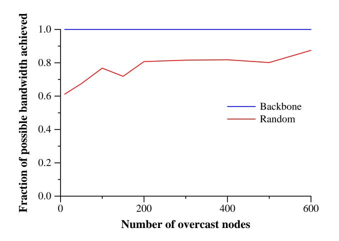
Overcast compared to a bandwidth optimal distribution tree.
