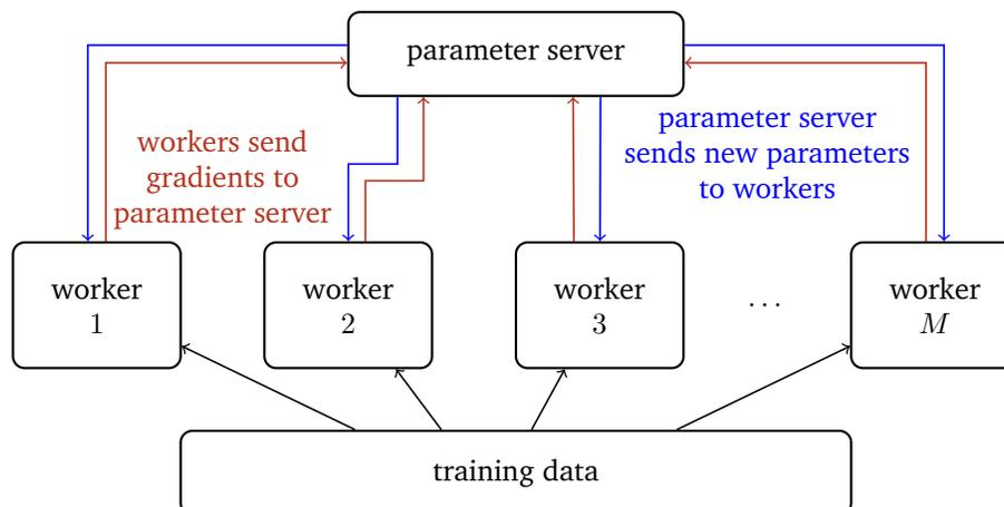
There are many ways to learn using a parameter server model, but one of the most common is **asynchronous distributed training**. This corresponds to the following algorithm.
