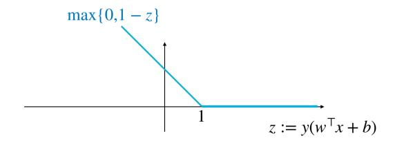
Hinge loss starts penalizing when functional margin falls below 1
