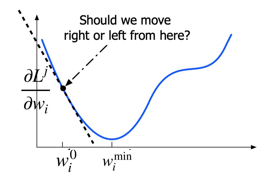
$$w_i^{t+1} = w_i^t - \alpha \frac{\partial L(y^j, x^j, w^t)}{\partial w_i}$$
