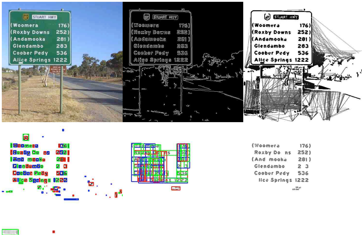
Figure 1: stages of the SWT algorithm. a) original image b) Canny edge detection c) stroke width detection d) connected components e) chaining f) final detected text
