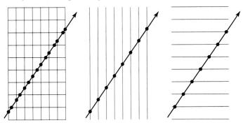
Instead of computing all values at once, an incremental DDA-type algorithm is preferrable in practice. In this problem, you will state concisely an efficient incremental algorithm to iterate over cells pierced by the advancing ray by effectively determining which of the x,y or z dimensions has the smallest t value. Assume that you can output a intersected cells by issuing the command output (i,j,k).
