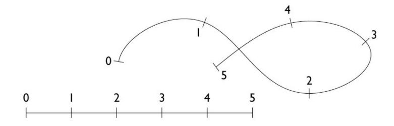
• 2D spline curves are parametric curves
