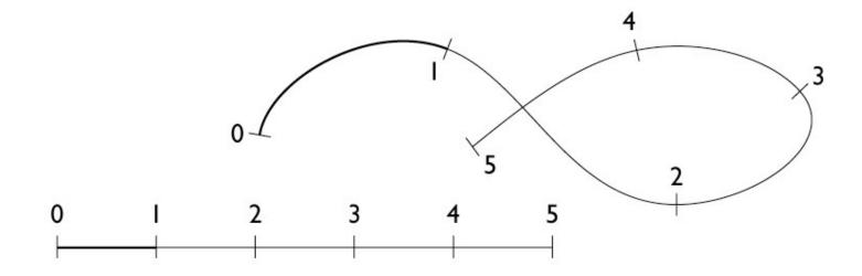
• 2D spline curves are parametric curves
