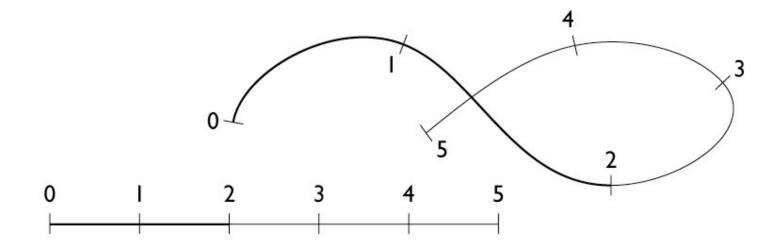
• 2D spline curves are parametric curves
