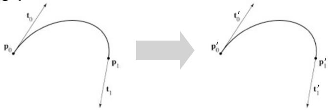
$$\mathbf{p}(t) = b_0 \mathbf{p}_0 + b_1 \mathbf{p}_1 + b_2 \mathbf{v}_0 + b_3 \mathbf{v}_1$$
