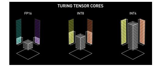
The GPU has so many cores that a photo of the chip is pointless. Instead they draw graphics like these to help you visualize ways of using hundreds of cores to process a tensor (the "block" in the middle) in parallel!
