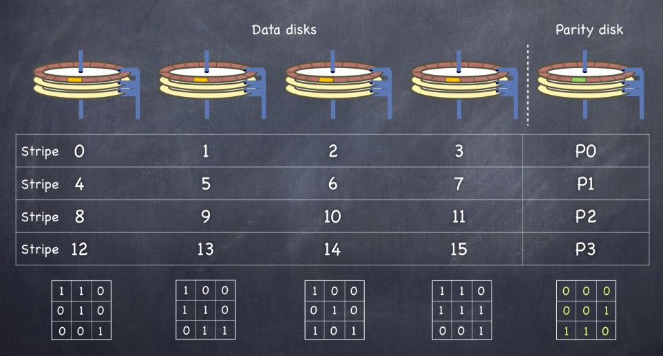
Disk controller can identify faulty disk
