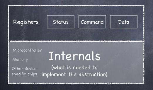
OS controls device by reading/writing registers
