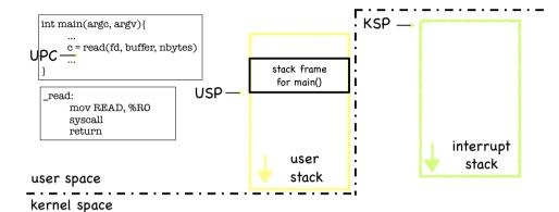
UPC: user program counter USP: user stack pointer KSP: kernel stack pointer
