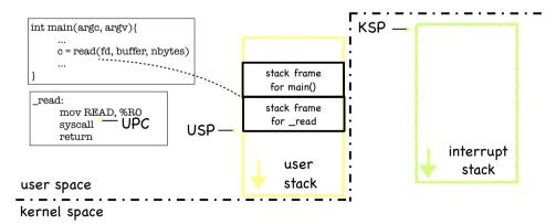
UPC: user program counter USP: user stack pointer KSP: kernel stack pointer
